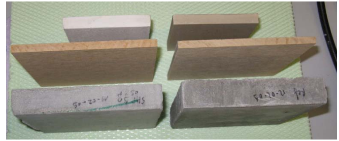
Figure 4: Optical picture of treated and untreated gypsum, FRC and mortar blocks after immersion in water and 30 minutes holding time.
