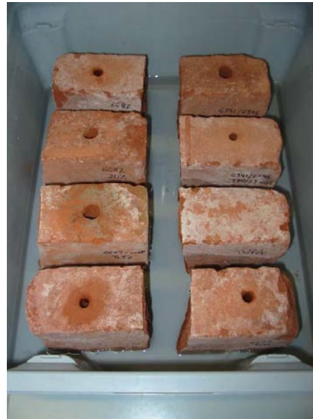
Figure 6: water uptake of clay bricks injected with 6682@ 60% or 7.5% as a function of immersion time. Picture showing the experimental set up to measure water uptake by capillarity rise.
